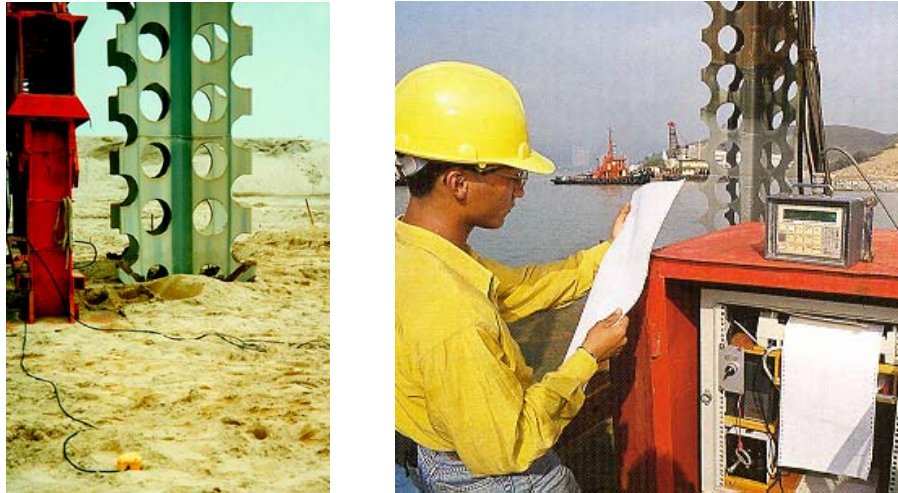
Fig. 11. Measurement of ground vibrations with the aid of a geophone (foreground) during compaction and monitoring of resonance compaction.
