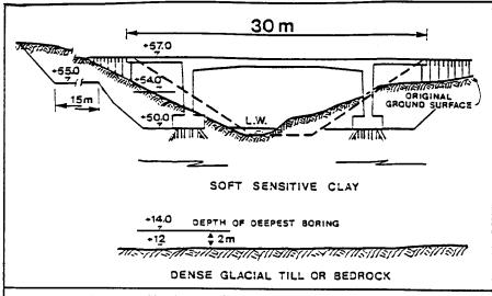
Longitudinal section of bridge and foundations
