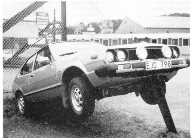
Fig. 1 The car with its front suspended by the pile hitting it from below
