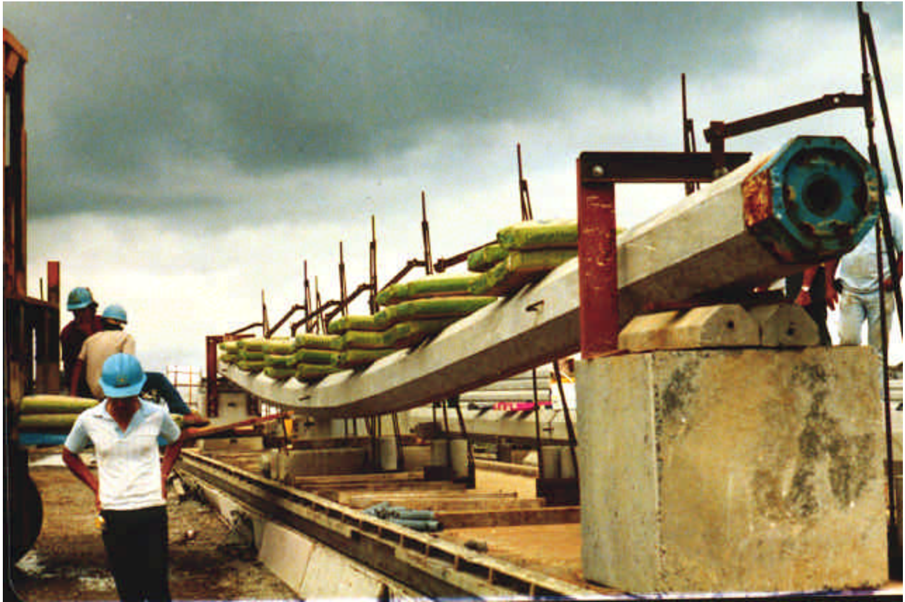
Bending of a pile segment for testing the efficiency of a center pipe probe Courtesy of F. C. Clemente, 1976
